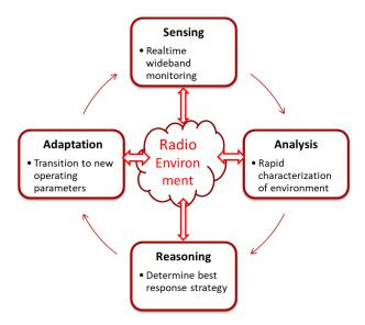
The cognitive RAN seeks to optimize radio performance continually by adapting modulation and demodulation schemes based on specified cost functions. This approach utilizes deep learning methods to allocate resources optimally, resulting in personalized waveforms for each device entering the network.
